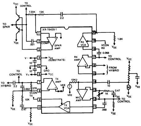
Figure 1. Typical Application Schematic
