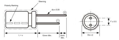
Drawing is representative of parts as supplied in bulk or straight lead format, please see taping specification for details on taped format packaging.
