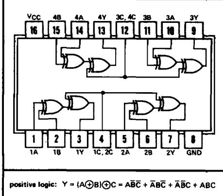
$$\text{positive logic: } Y = (A+B) \oplus C = \bar{A}\bar{B}C + \bar{A}B\bar{C} + A\bar{B}\bar{C} + ABC$$
