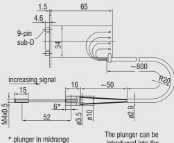
The plunger can be introduced into the sensor from both ends.
