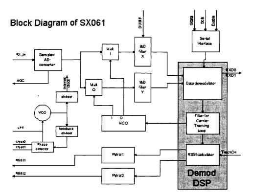
The SX061 also generates an AGC output. This AGC signal is used to control the amplification of the amplifier in the Radio Unit. This guarantees an optimal quantization of the incoming signal.
