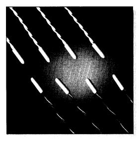
The PVC tip encapsulation allows the use of a standard size thermistor chip for applications where a small, consistent size is needed. Typically, an epoxy coated thermistor would be approximately .015" to .020" greater in diameter than a PVC tipped device. This type of construction is ideal for applications where the sensor must be placed inside a long, thin tube.
