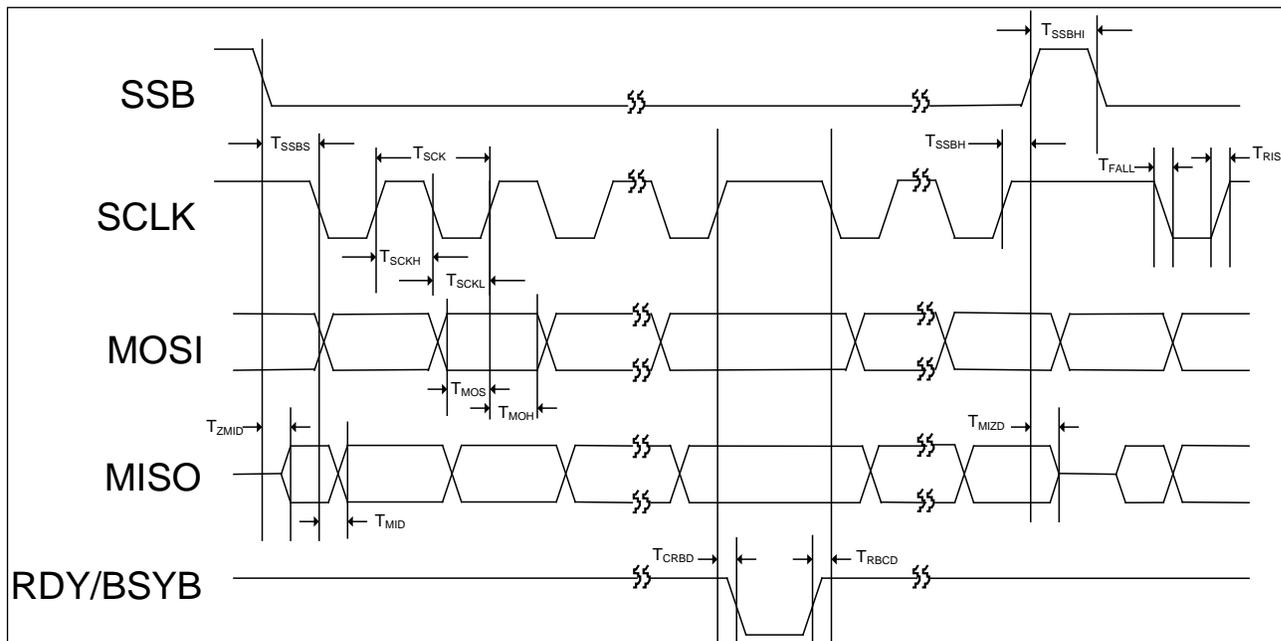
Figure 11-2 SPI Timing
