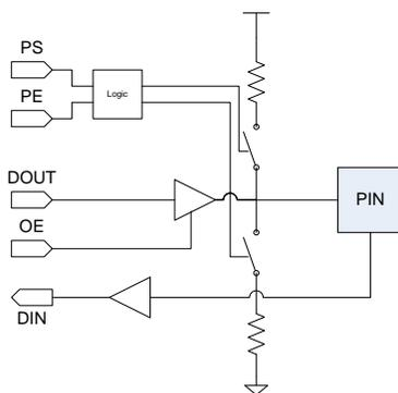
Figure 6-1 GPIO Structure
