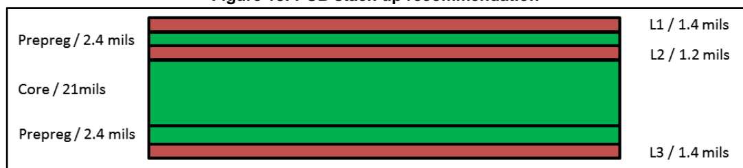
Figure 18: PCB stack-up recommendation
