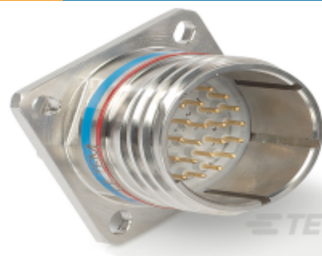
TE Model / Part #YDTS20F09-35ANV001 D38999: Square Flange, 9-35 insert
