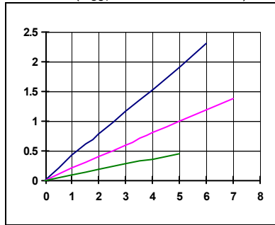
Output Voltage vs. Sense Current ( R_{OUT} = 100 \Omega at 100 KHz)
