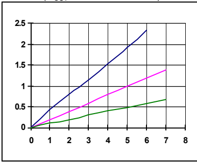
Output Voltage vs. Sense Current ( R_{OUT} = 100 \Omega at 10 KHz)
