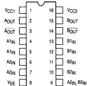
Pin assignment is for Dual-in-Line Package.
