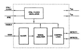
The MX633 is a low cost, low power device that uses signal processing techniques to detect audible tone signals such as Dial, Ringing, Busy and other conditions found when placing a call throughout the world's telecom systems. Detection of these call progress stages is essential to the proper operation of automatic calling products.
