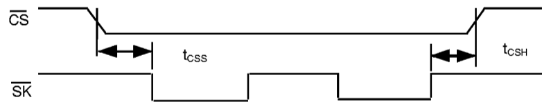
Figure 4 Timing Chart for t_{CSS} and t_{CSH} when \overline{SK} is "H"
