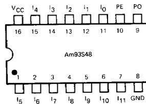
Note: Pin 1 is marked for orientation.
