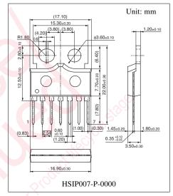
Note) The package of this product will be changed to lead-free type (HSIP007-P-0000B). See the new package dimensions section later of this datasheet.
