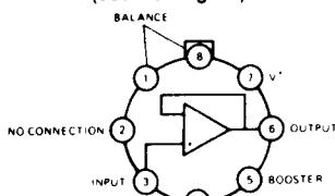
NOTE: Pin 4 connected to case
