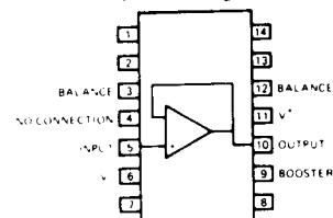
NOTE: Pin 6 connected to bottom of package
