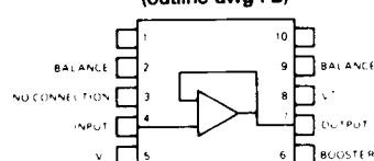
NOTE: Pin 5 connected to bottom of package
