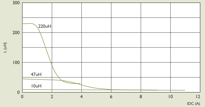
SCDS125, INDUCTANCE vs. IDC CHARACTERISTICS
