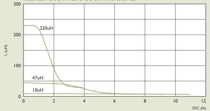
SCDS125, INDUCTANCE vs. IDC CHARACTERISTICS
