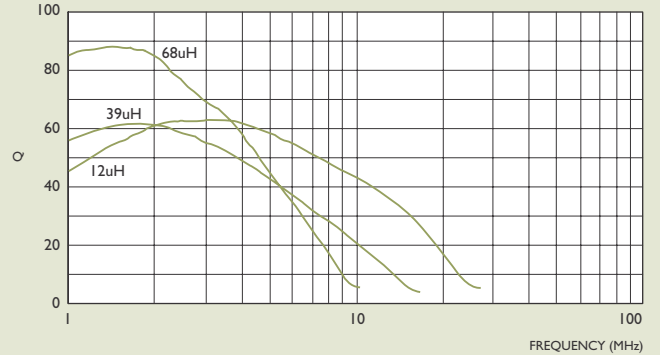
NL453232, Q vs. FREQUENCY CHARACTERISTICS
