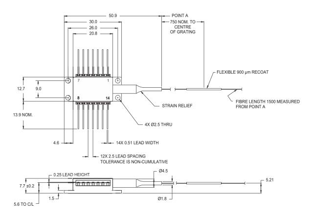
Dimensions Diagram 250 µm Bare Fiber Type A Wiring (Specifications in mm unless otherwise noted.)
