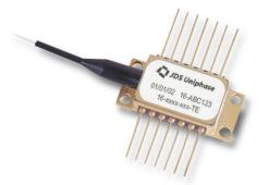
The JDS Uniphase 1600 Series is a new product line of 960 nm pump modules for use in L-band EDFAs in both long haul and metropolitan area fiber networks. These pumps can be applied in wideband EDFAs in a dense wavelength division multiplexing (DWDM) fiber optic network. They can also be used in a L-band, single channel or low channel count, narrow band erbium doped fiber amplet.
