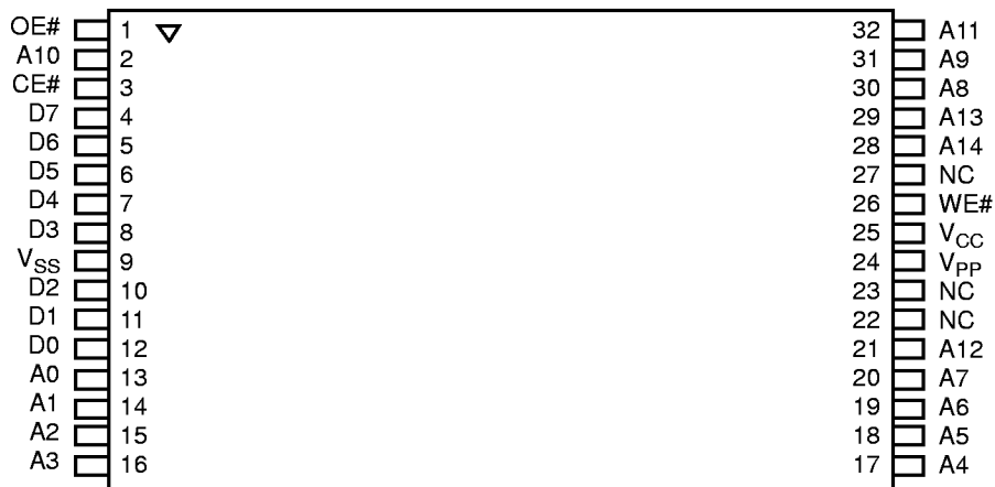
32-Pin TSOP—Reverse Pinout
