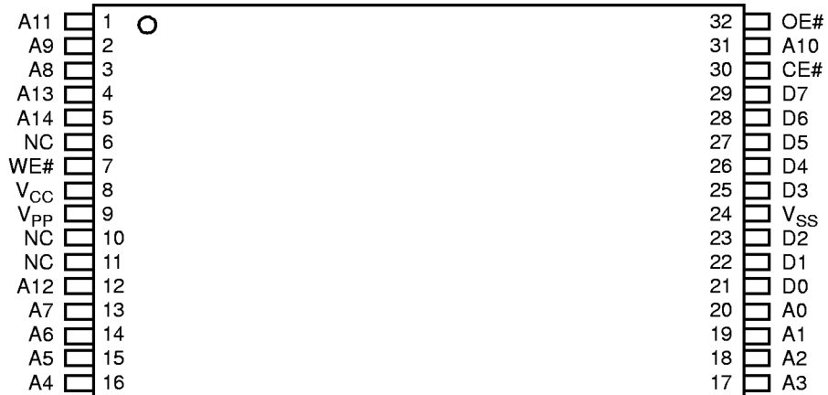
32-Pin TSOP—Standard Pinout
