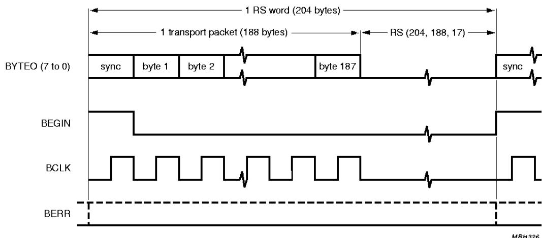
Fig.6 Output Interface timing.
