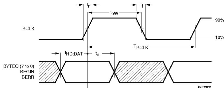
Fig.8 Output data timing waveforms.
