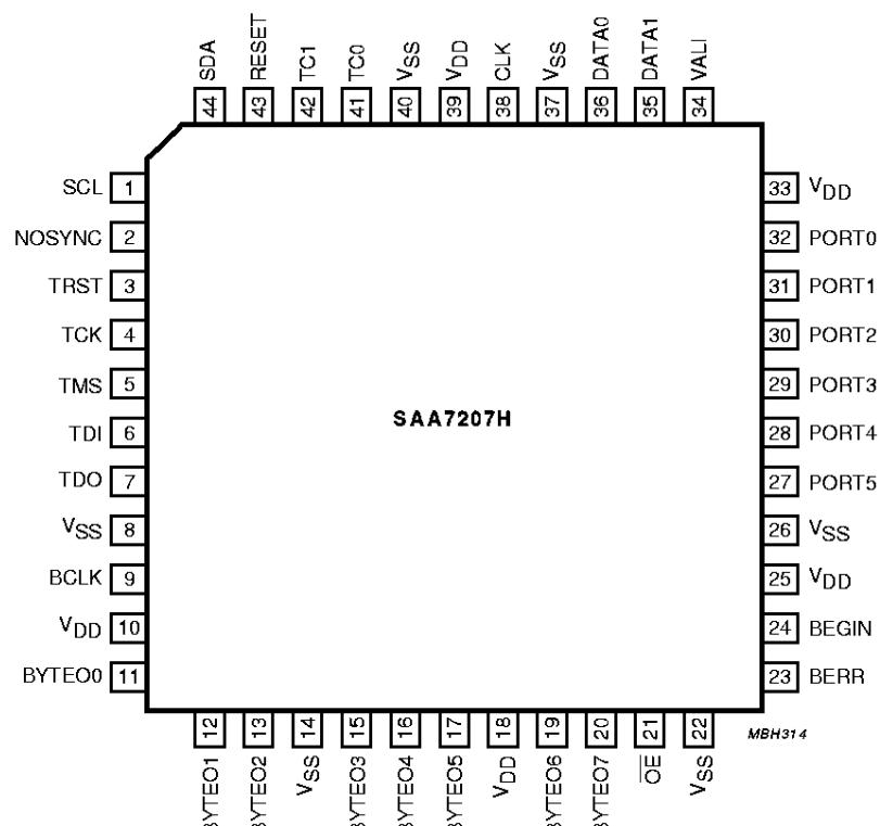
Fig.2 Pin configuration.
