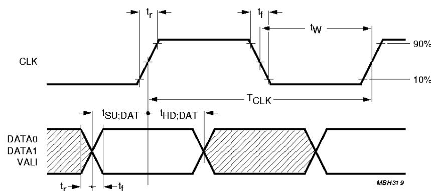
Fig.7 Input data timing waveforms.
