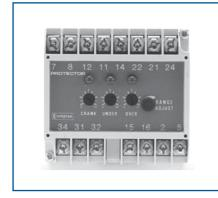
1mA analog output 3 adjustable setpoints Adjustable time delay Internal differential LED trip indication Automatic reset 3 single pole relays Magnetic pick up input
