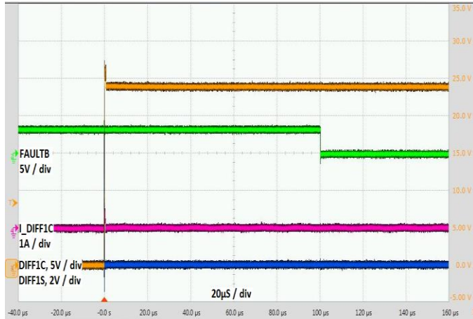
Figure 15. DIFF1C Short to 24V Vbus
