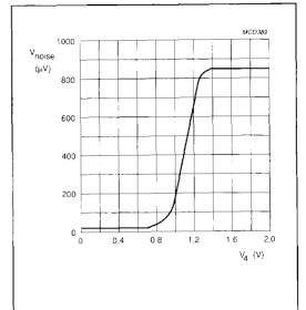
Fig.4 Noise output voltage as a function of DC volume control.
